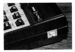
A DIP switch on the 41's exterior can temporarily disable the internal time module while the versatile adapter is plugged in. The module can be made "invisible" without the loss of time, date or accuracy factor.
