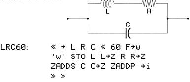
The name, LRC60, tells you that you must key in the L, R and C values in that order and that they will be combined at 60 Hz. The result will be returned in 'Re+i\*IM' format. Note that if you were to omit i, this program it could be used to generate algebraic objects.
