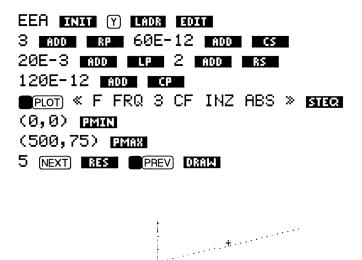
Note that flag 3 is cleared before the call to the calculation routine (INZ in this case). Flag 3 is an optimizing feature of the ladder analysis tools. When it's set, the circuit list is not "re-crunched" before the calculation, thus speeding up multiple calculations on the same circuit. Clearing flag 3 therefore forces a "re-crunching" of the circuit – necessary because you want to evaluate it each time at a different frequency.
