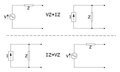
The conversions are trivial but useful for converting source configurations between series and parallel. For example, to reduce the following parallel-voltage circuit to its equivalent series-voltage and impedance:
