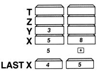
In a similar manner, if the wrong **function** key was pressed, a user can recall LAST X, reverse the function, and then proceed with the correct operation.
