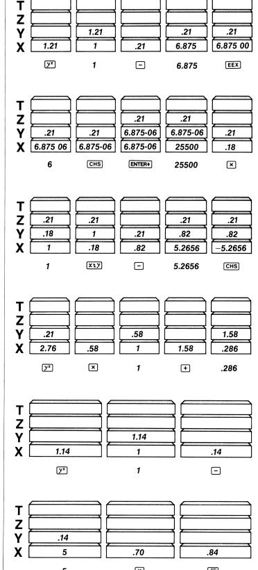
The HP RPN system enabled this calculation to be attacked and worked in the same order as if it were worked longhand with pencil and paper.
