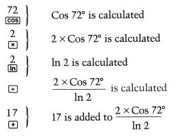
The function keys always follow directly the numbers to be operated on, whether the function is a single-argument function (Cos, ln) or a two-argument function ( $\times$ ,  $\div$ , +).
