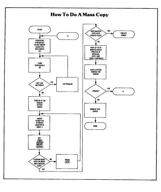
**Note:** Since MSCOPY destroys the data on all cassettes except the one in the first drive, make sure that you know which drive is the first drive in the loop before attempting to execute MSCOPY. When you execute MSCOPY, the busy light on the first drive will flash for 10 seconds before the copy process begins. This gives you a last chance to save your master cassette if it is in the wrong drive. If the
