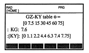
Here the GZ table (GZ curve) for KG = 7.6 metres and KY values as given is calculated. The table is calculated in the interval [0 75], for every  $2.5^{\circ}$  between 0 and  $60^{\circ}$ . The last row gives the max GZ with corresponding angle. The value of KG is stored for future reference (KG option in user menu).
