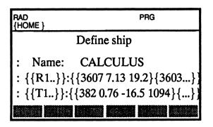
Next picture is the matrix writer where the table will be constructed. The data given so far is the name of the ship, data for rooms (R) and tanks (T) in double lists  $\{\}\}$ . For rooms the volume, KG and KGL are put into the list. For new rooms the corresponding data are put into a new list {}. For tanks the same data are given in addition to moment of inertia for calculating the effect of free surface. For two rooms and two tanks the double lists may look like this:
