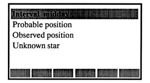
If you now press ENTER, the input form for interval to apparent midday is displayed, which calculates time and current position at midday.
