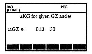
Here the change in KG if the change in GZ for  $30^{\circ}$  is 0.13 metres is calculated. The problem might be to calculate the weight to be moved when the GZ at given angle is given.
