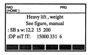
The example calculates the change in KG and GZ arm when the distance to the top of the boom from the centre of mass is 12.2 metres. The distance from the mast to the top of the boom is 15 metres and the weight is 200 tons. Displacment 15000 tons and ballast 331 tons with centre of mass 6 metres form the centre line. New GZ curve may be calculated (with new KG) and the heeling angle may be found for the calculated GZ arm.
