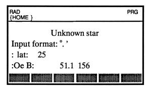
This example calculates the declination of a star with a corrected elevation of  $51.1^{\circ}$  and a gyro bearing of  $156^{\circ}$ . The latitude is 25 N. The output is negative, which indicates a southerly declination.
