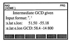
The example calculates the intermediate position at a distance of 800 nmi from Belle Isle along the great circle to Rock All.
