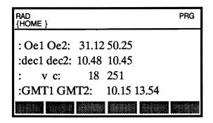
This example calculates observed position for two observations made at 10.15 GMT and 13.54 GMT. The estimated position is 50.42 N 26.19 W, and declination, corrected elevations and hour angles are given.
