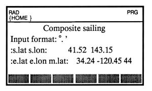
The example shows composite sailing from Korea to Los Angeles with 44 N as the maximum latitude. The output data shows course, distance and end position for the first great circle (GC 1), the parallel at 44 N and the second great circle (GC 2). The last row in the table shows the total distance, the direct great circle distance, the rhumb line distance and the deviation in distance from the direct great circle route.
