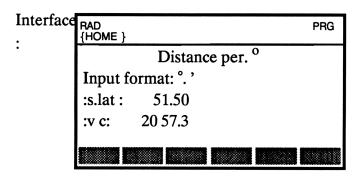
This example calculates distance per degree change of course for a passage from 51.5 N at a speed of 20 knots and a course of  $57.3^{\circ}$  (Belle Isle/ Rock All).
