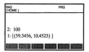
In the example TOL is the distance around the Way-point indicating the arrival (100 m) and the sailing goes to the Way-point 59.3456 N 10.4528 E. If several points are used they are put into a list in the same way {(59.2345,10.2567) (59.5648,10.3789)}.
