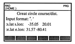
The above example calculates distance, start course, end course and vertex point for the great circle route from 35.05 S 20.01 E (Cape Agulhas) to 31.57 N 80.41 W (Savannah) using degrees and minutes input format. The answers are gathered in a list and can be separated using  $PRG/OBJ \rightarrow DROP$  on the calculator keyboard.
