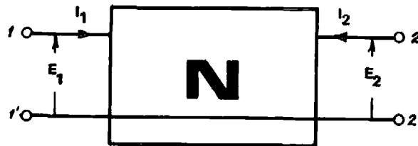
Figure 4-3.1 Two-port network conventions.
