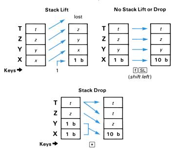
Typically, one-number functions (as defined in the previous section) result in no stack movement, while two-number functions *usually* result in a stack drop.
