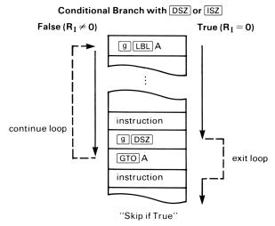
The value in  $R_I$  is interpreted according to the current complement mode. It can be positive or negative, in integer or floating-point format. The instructions  $\boxed{\text{DSZ}}$  and  $\boxed{\text{ISZ}}$  do not affect the status of the carry and out-of-range flags.
