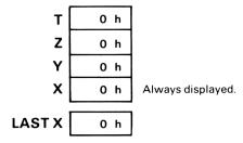
The number that appears in the display is the number in the X-register—unless the calculator is in Program mode (**PRGM** annunciator displayed).
