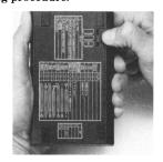
Grasp the outer edge of the battery compartment door, then tilt it up and out of the calculator.
