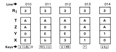
Line 012 does a checksum of the contents of the register currently addressed by  $R_{\rm I}$ , and line 013 adds this checksum to the least significant part of the checksum. Lines 014 to 017 add in the carry bit from the previous add to the most significant word of the checksum.
