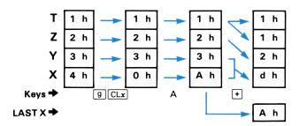
As you can see, when an arithmetic operation is performed with operands ( $A_{16}$  and  $3_{16}$ ) in the X- and Y-registers, the stack drops and the result ( $D_{16}$ ) is left in the X-register.
