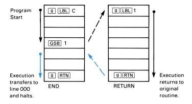
**Nesting.** Subroutine "nesting"—the execution of a subroutine within a subroutine—is limited to a nest of subroutine returns four levels deep (not counting the main program level).
