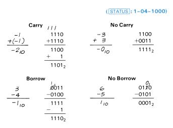
The Carry Flag During Addition. The carry flag (flag 4, C annunciator) will be set whenever a binary addition results in a carry "out of" the most significant bit. If an addition does not result in such a carry, the carry flag is cleared. This is the same for all complement modes.
