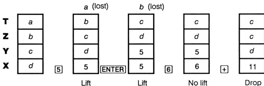
**ENTER** replicates the contents of the X-register into the Y-register. The next number you key in (or recall) *writes over* (instead of lifting) the copy of the first number left in the X-register. The effect is simply to separate two sequentially entered numbers.
