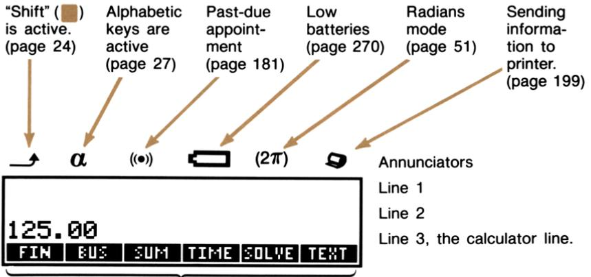
Menu labels for the MAIN menu. To display the MAIN menu, press the
