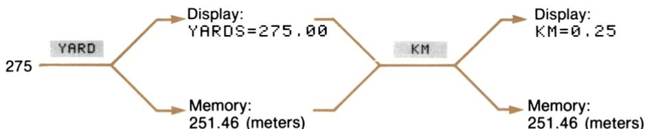
**Figure 3-3. How the HP-19B Does Unit Conversions**
