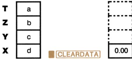
Because of the automatic movement of the stack, it is *not* necessary to clear the stack before starting a calculation. Note that if an application menu is currently displayed, pressing **CLEAR DATA** also clears the application's variables.
