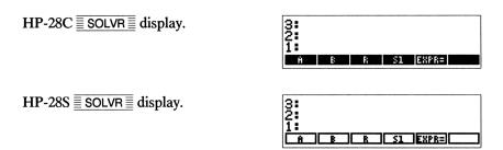
Both of these screens include the Solver variables A, B, B, R, ES, SI, and EXPR= . The HP-28C displays Solver variables in gray on a black background. The HP-28S prints Solver variables in black on a gray background.
