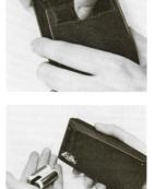
Turn calculator over and turn power on to assure proper battery installation. If the display does not light make sure the battery pack is correctly placed in calculator.
