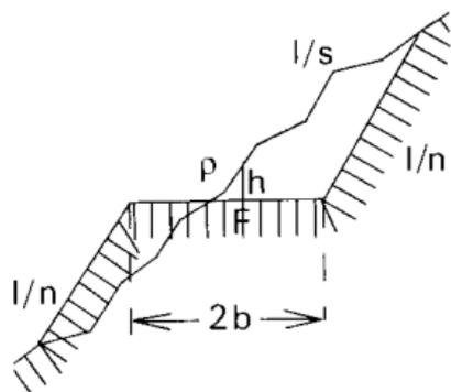
Which of  $A_1$  and  $A_2$  is cut and which fill depends on whether  $p$  is to the right or left of centre line F
