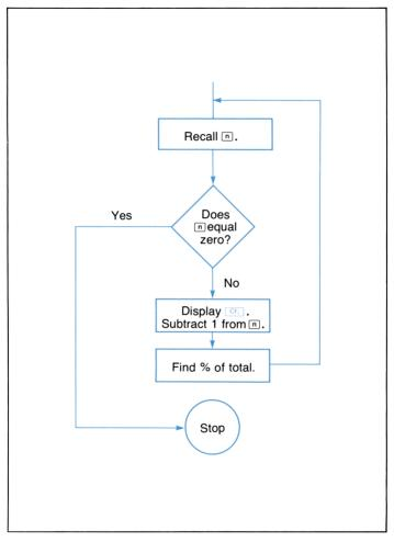
The n register has been counting the number of CF, entries, so we can use it in the decision-making process. Each time we recall a CF, entry, the contents of the n register are automatically decreased by 1.00. When n is decreased to zero, the program stops.
