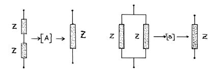
Just as in the editing routine, these keys speak whatever language you are currently working in–Polar, Rectangular or Physical. You load up the stack with four numbers; the top two represent one complex impedance; the bottom two, another. The [A] key will combine these impedances in series (recall that impedances add linearly when in series), while the [a] key will assume they are in parallel (and therefore add them inversely).
