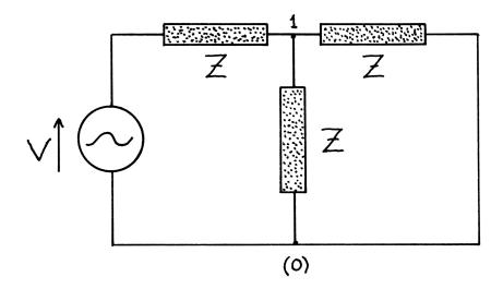
Here you see a sinusoidal voltage source and three impedances. The point labelled "1" in the circuit is called a node, because it is the junction of three (3) or more elements. In this program, you can name other points as nodes also, but you HAVE to name all points that connect three or more elements.
