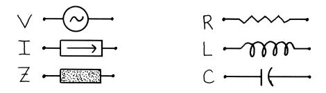
Keep in mind that you can always combine an R and either an L or C into a Z. This saves time and represents just one element in the circuit, rather than two (and this saves memory for the calculator).
