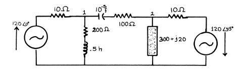
So if you have a circuit such as the one above, and you want to find the input impedance at nodes 1 and 2, do the following:
