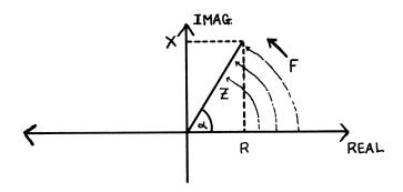
How do we know this? Well, when you measure voltage, current or power with meters, you are measuring only the real portions of those quantities; if you trace the behavior of ONLY the real portion (i.e. the x-component) of a complex number as it rotates around the axis, it WILL describe a sinusoidal pattern (Aha)!
