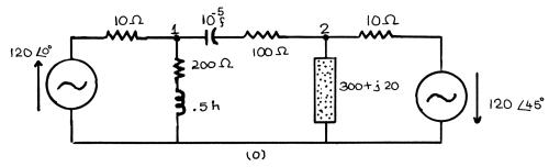
And suppose that, for more laughs, you wanted to calculate the voltages at node 1 and node 2, and the currents through the (300 + j20) impedance and the .5-henry inductor.
