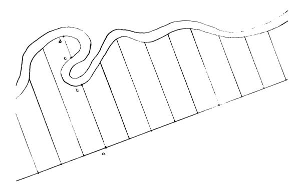
As you can see from the diagram above, as we make the fourth measurement from the left, we have to go across a fold in the creek. In this case we simply use the sum of the two segments (from a to b and from c to d).
