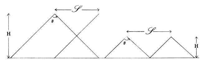
In the diagram above, H is the nozzle height, S is the nozzle spacing, and  $\theta$  is the spray angle. The formula for the overlapping case is:
