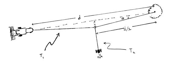
The distance x can be varied by adjusting the slack in the main cable  $(T_1)$ , and the distances d and x will determine the relationship between  $T_1$  and  $T_1$ . Of course, x will increase as the cable stretches or the stuck machine begins to move.
