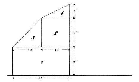
The area of one half of the front of the barn is divided into two rectangular sections and two triangular sections in the figure above. We can sum the areas of these sections and multiply by 2 to get the total front area. Multiplying this area by the length will give us the volume.
