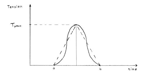
For our purposes, the triangular spike function shown with hatched lines will be a good enough approximation to the impulse function. The impulse is equal to the area under the curve which is in turn equal to one half the time interval multiplied by the height of the pulse, and the height of the pulse is just the peak tension. (The peak tension is what we are ultimately interested in.)
