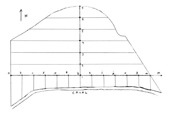
Now suppose we want to plant a certain number of acres in a field of arbitrary shape. Referring to the figure above, suppose we pick out landmarks and plant the initial land along a line between points  $\underline{a}$  and  $\underline{n}$  (rows running E-W). After we have planted to the canal, we go back to the other side of the land and we want to know how far to plant to the North. We might be interested in how far on the map in 1/32 in., how far in the field in ft., or how many rows.
