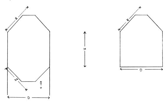
The level will be measured from the bottom of the bin where the lower cone is truncated a distance T above its apex. Measurements will be in inches.
