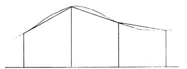
(6) As in the diagram above, we will use the areas of trapezoids as approximations. For each segment, calculate the area on the planted side with the following keystrokes.
