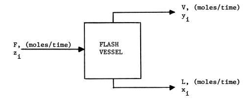
A five component mixture of hydrocarbons is fed to a steady-state flash vaporization giving product equilibrium at 270°F and 50 psia. The details are given below:
