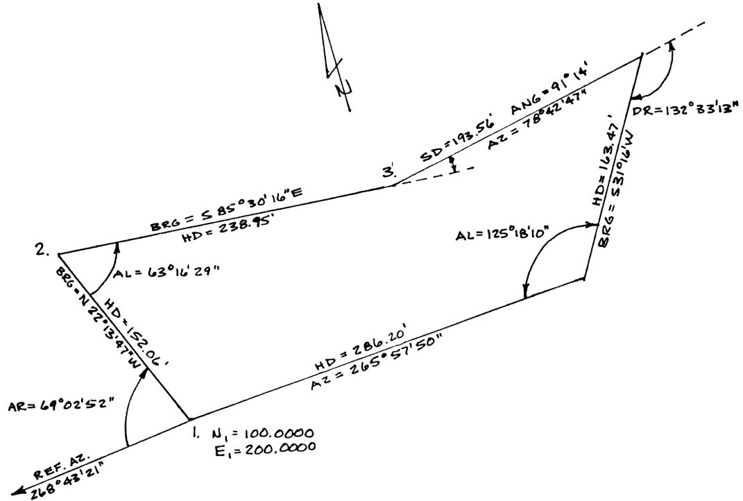
Perform traverse computations with the data given in the sketch and prepare the data for adjustment.
