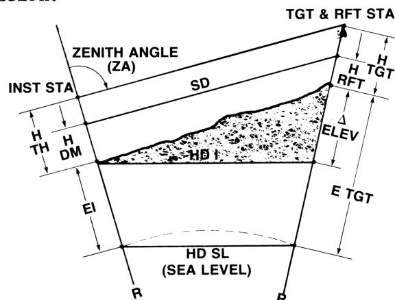
Using the values shown in the example, reduce the slope distance to a horizontal distance.
