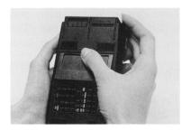
3. Remove the batteries from the battery holder.
