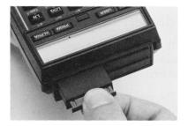
The information in an extended memory module is lost when the module is removed from the computer. You can lose all data in two extended memory modules even if you remove only one of the two modules. To avoid this, observe the following rules when choosing which of two modules to remove.
