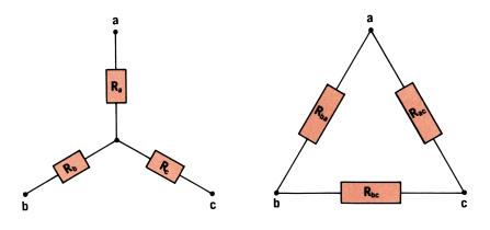
$$\begin{split} R_{ab} &= \frac{R_a R_b + R_b R_c + R_c R_a}{R_c} \\ R_{bc} &= \frac{R_a R_b + R_b R_c + R_c R_a}{R_a} \\ R_{ca} &= \frac{R_a R_b + R_b R_c + R_c R_a}{R_b} \end{split}$$
