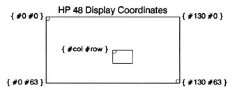
The built-in commands  $PX \rightarrow C$  and  $C \rightarrow PX$  convert between user coordinates, such as (x,y), and pixel coordinates. The Tool Library commands  $PX \rightarrow R$  and  $R \rightarrow PX$  simplify the translation between pixel coordinates and loop indices or calculation results.
