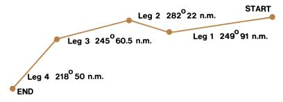
Winds for legs 1 and 2 – 230 degress @ 30 knots (true). Winds for legs 3 and 4 – 300 degrees @ 20 knots (true). Fuel consumption 8 gal/hr, TAS 105, magnetic variation 15 degrees E.
