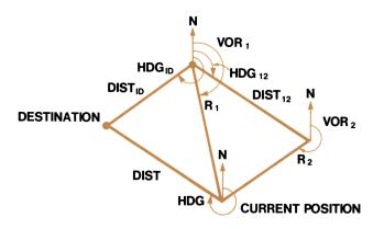
$$D_{1} = \left| \frac{DIST_{12} \sin(R_{2} - HDG_{12})}{\sin(R_{2} - R_{1})} \right|$$
