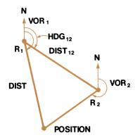
$$DIST = \frac{DIST_{12} \sin(R_2 - HDG_{12})}{\sin(R_2 - R_1)}$$
