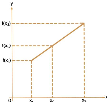
2. This program also evaluates for interpolation argument  $x$  the Lagrangian interpolating polynomial  $P_2(x)$  of degree two passing through the points  $(x_0, y_0), (x_1, y_1), (x_2, y_2)$ .
