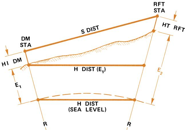
$$H \text{ Dist} = \left[ \sqrt{\frac{(S \text{ Dist})^2 - (E_2 + HT \text{ Rft} - E_1 - HI \text{ DM})^2}{(R + E_1 + HI \text{ DM})(R + E_2 + HT \text{ Rft})}} \right] [R + E]$$
