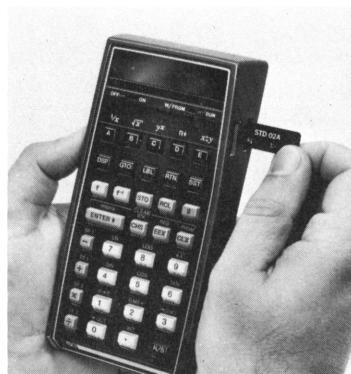
When the motor stops, remove the card from the left side of the calculator and insert it in the upper "window slot" on the right side of the calculator.
