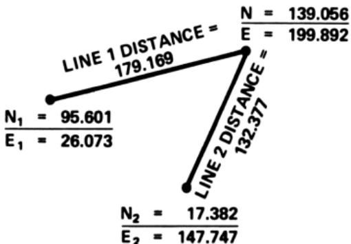
NOTE: Computed solution is always clockwise from point 1 to 2. For alternate solution, start at Point 2.
