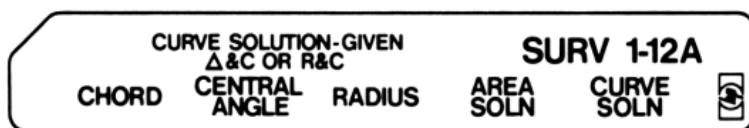
Given the chord length and either the central angle or radius, this program computes four remaining parameters plus the sector, segment and fillet areas.
