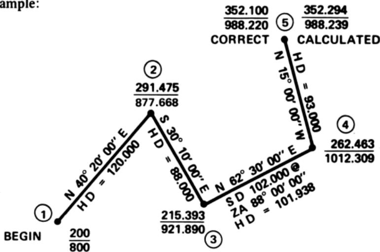
In this example, the Bearing Traverse program is used until the calculated ending coordinates are established. The Closure for Field Angle & Bearing Traverse program is then loaded and the closing coordinates are entered ( $N = 352.100$  and  $E = 988.220$ ). From there, the remaining closure information can be obtained -- see instructions for the Closure program (*Surveying 1-3A*).
