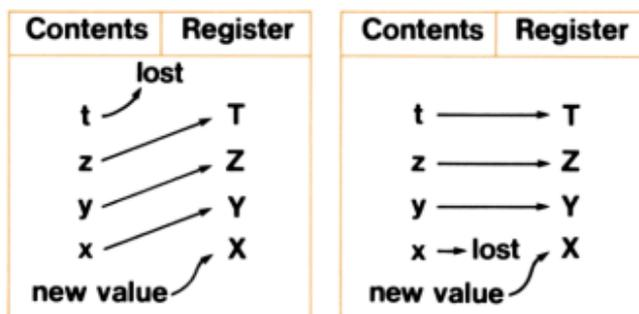
**Lift Disable Keys:** **R/S** in a program if the program has just put a new number in the X register from program memory; **CLX**, **ENTER↑** at any time.
