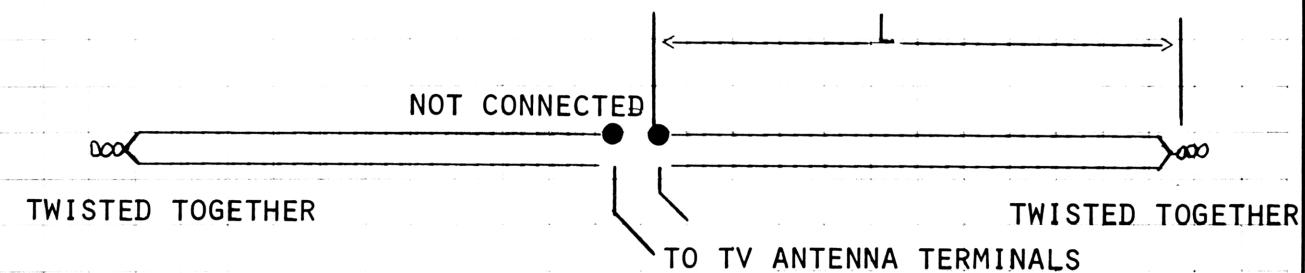
Use ordinary lead-in (flat) wire. Twist wire together as indicated above after cutting as shown. Connect to TV set antenna terminals. Adjust direction of the antenna for the best picture. Leave gap at the top, as shown. Tape bare wires.
