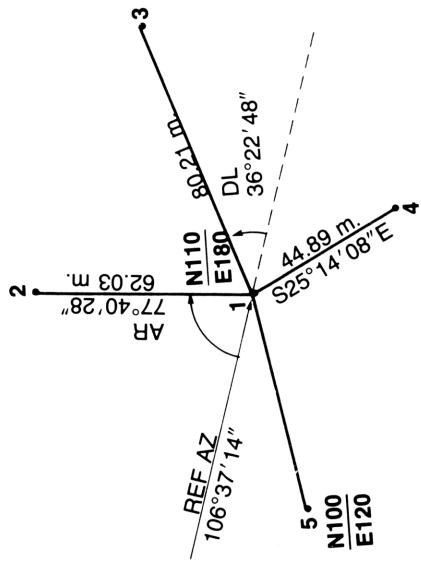
Starting from point 1 with coordinates N110, E180, calculate the sideshots shown in the figure above.
