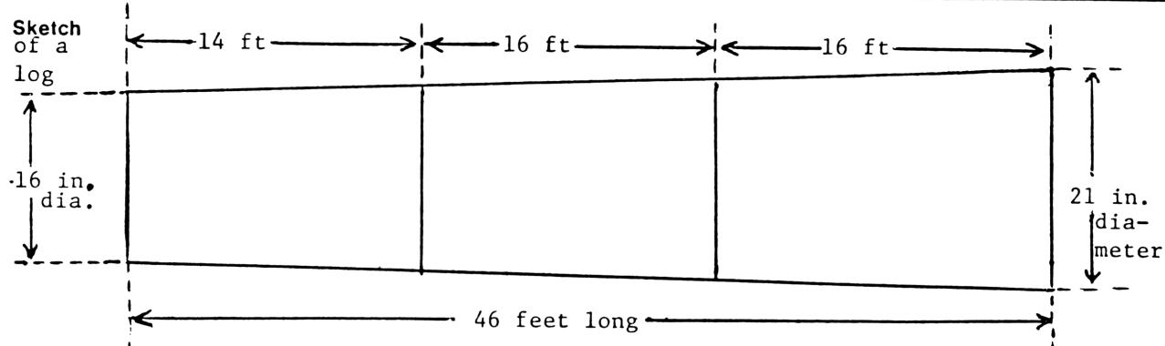
**Sample Problem(s)** Find the recoverable and cylindrical board feet in a log that is 46 feet long with end diameters of 16 and 21 inches,
