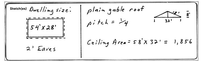
Sample Problem(s) FOR THE DWELLING WITH THE ABOVE DIMENSIONS, FIND RAFTER LENGTH, ROOF AREA, NUMBER OF SQUARES, MATERIAL COST, LABOR COST, TOTAL COST OF ROOF, AND, CONTINUING FROM <u>LUMBER ESTIMATE</u> (1054D). FIND TOTAL COST AND TOTAL MATERIAL AND LABOR COSTS FOR THE ROUGH LUMBER AND ROOF.
