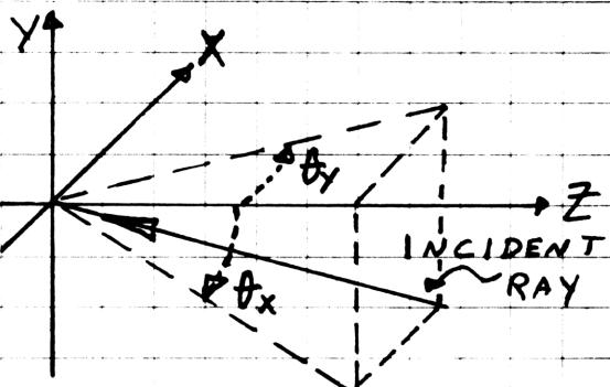
Sample Problem(s) a) FOR A PARABOLIC MIRROR WITH A FOCAL LENGTH OF 50 CM FIND THE COORDINATES OF A REFLECTED RAY IN AN IMAGE PLANE 50 CM FROM THE MIRROR WITH THE MIRROR TILTED  $-1^\circ$  AND WITH THE INCIDENT AT AN ANGLE OF  $\theta_x = 0.5^\circ$ ,  $\theta_y = 2^\circ$  HITTING THE MIRROR AT  $X_m = 5$ ,  $Y_m = 6$ .
