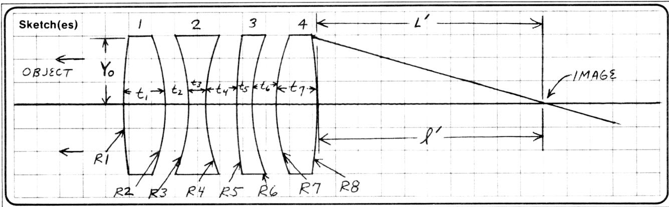
**Sample Problem(s)** (FROM REFERENCE 1 CH. 88) FIND THE ABERRATIONS OF A THREE LENS PHOTOVISUAL OBJECTIVE WITH PARAMETERS: LENS 1  $N_c=1.51358$ ,  $N_d=1.5160$ ,  $N_f=1.52167$ ; LENS 2  $N_c=1.53447$ ,  $N_d=1.5376$ ,  $N_f=1.54516$ ; LENS 3  $N_c=1.57968$ ,  $N_d=1.5833$ ,  $N_f=1.59219$ ;  $Y_o=.25$ ;
