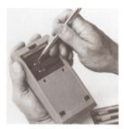
See if the battery connector springs on the calculator have been inadvertently flattened inward. If so, bend them out and try the battery again.
