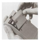
6. Insert the bottom of the battery door behind the retaining groove and close the door.
