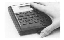
To remove the module, grasp the lip on the bottom of the front edge of the module and pull the module straight out of the port. Install a blank module in the port to protect the contacts.
