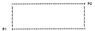
The scaling points P1,P2 have a different default depending on the plotter module, plus they may be manually set by controls on the plotter. Thus what makes sense to one plotter may be garbage to another.
