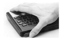
To remove the module, use your fingernails to grasp the lip on the bottom of the front edge of the module and pull the module straight out of the port. Install a blank module in the port to protect the contacts inside.
