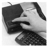
2. Remove the port cap that is in the lowest numbered unused port. If you must remove a memory module, always remove one from the highest numbered port. (If you remove a memory module, make sure the HP-41C has enough memory allocated to data storage registers—executing SIZE 064 will ensure this.)
