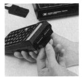
3. Insert the printer interface module into the empty port as shown. Push it into the calculator until it snaps firmly into place.
