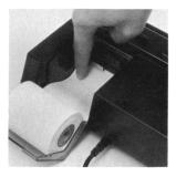
Press the paper advance key and hold it down until the paper passes the top of the plastic tear bar.
