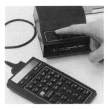
2. Pull the printer interface module straight back until it is free from the port. Do not pull on the cord.
