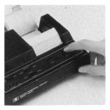
5. Drop the roll of paper into the paper well, close the cover, and press PRINT two or three times. (If you ran out of paper during the execution of a program, press (R/S).) If the paper is feeding properly but no printing appears when you print, the paper may be inserted backwards. The paper is chemically treated and will print on only one side.
