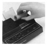
Before inserting the new roll of paper into the printer, discard the first two turns to ensure that no glue, tape or other foreign matter is on the paper. Make sure that the leading edge of the paper is straight, not crooked or jagged. A short, sharp crease on the leading edge may aid in the loading of the paper.
