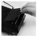
6. Secure the door by pressing it gently while sliding the two battery door latches outward.
