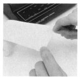
3. Temporarily place the paper roll in the paper roll cover. With your finger, push the leading edge of paper into the slot near the bottom of the paper well. Continue pushing until the paper can be pushed no further into the print mechanism.
