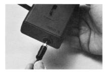
When using the video interface, the switch on the switch box should be set to INTERFACE. When viewing normal television programs, the switch should be set to TV.
