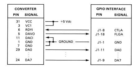
The second installation provides one-way communication from the GPIO interface to the converter. The converter uses the default values for its control registers. (The GPIO interface must have bits 4 and 0 of register 3 equal to 1—FLGA and CTLA negative-true—and bit 0 of register 8 equal to 1—Output Enable A; other registers use their default values.)
