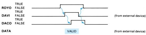
**Logic System.** The converter uses positive logic or negative logic for the data buses and for the handshake lines—each specified independently by control register R02-5,4.
