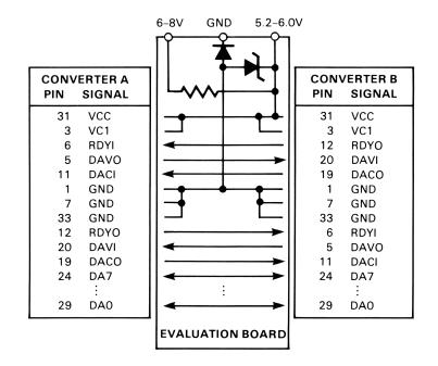
This connection can also be used to check the operation of two converters. You can join the interconnected converters in the same HP-IL system, then send data to one converter and retrieve it from the other. (Refer to appendix A.)
