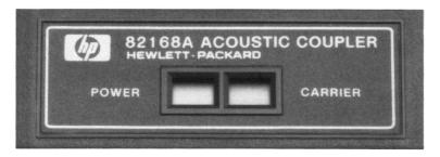
**POWER Indicator.** The POWER indicator shows whether or not the coupler is powered up. When the coupler is powered up, the POWER indicator will become dark red. When it is powered down, the POWER indicator will become pale red.
