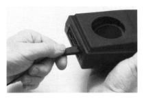
To maintain long battery life, it is recommended that you always fully charge the battery pack and let it fully discharge before you recharge it. Otherwise, the charging capacity of the pack will be reduced.
