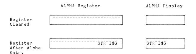
As illustrated above, the display shows the contents of the ALPHA register, beginning with the leftmost non-null character. The beginning of the string is left-justified in the display (or scrolled left if it is followed by more than 11 characters). If nulls occupy one or more of the leftmost positions in the register, those **leading** nulls are ignored in the Alpha display. When a null is preceded on the left by any non-null characters, it is displayed as the overbar (<sup>-</sup>) character.
