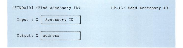
[FINDAID] allows the HP-41 to locate a device of a specific class or type which you specify with a number in the X-register. If the number is positive, [FINDAID] searches the loop, starting with the primary device, until it finds a device whose accessory ID matches the number (integer part) in the X-register. If such a device is present, its HP-IL address is returned in the X-register.
