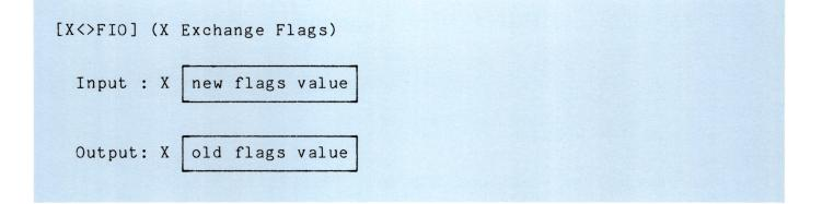
[X<>FIO] exchanges the current number in the X-register with the decimal equivalent of the binary number represented by flags 00 through 07, which enables you to test individual bits in an eight-bit byte. Flags 00 through 07 are reset according to the value in the X-register when you execute [X<>FIO]. ([X<>FIO] is identical to [X<>F] in the Extended Functions/Memory module.) Each of the 8 flags can represent one binary bit--flag 07 is the most significant bit, flag 0 the least significant bit.
