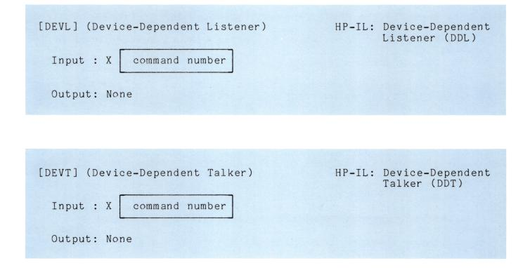
[DEVL] and [DEVT] send the Device-Dependent Listener and Device-Dependent Talker commands, respectively, according to the number in the X-register. The commands are sent to the primary device. The command number must be in the range  $-31 \leq n \leq 31$ . Numbers outside the allowed range will result in the DATA ERROR display.
