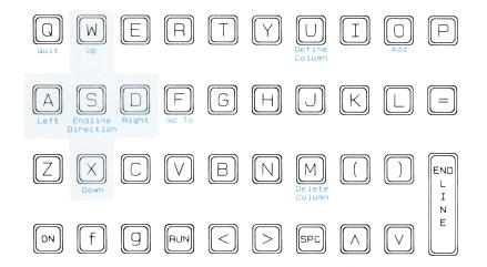
**The Direction Keys.** The direction keys are found in the cross on the keyboard diagram. You can use the direction keys in combination with the f key to move anywhere in the array. Once you get to the row and column you want, you can examine the contents of the element at that location and/or modify it.
