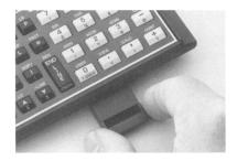
To remove the module, use your fingernails to grasp the lip on the bottom of the front edge of the module and pull the module straight out of the port. Install a blank module in the port to protect the contacts inside.
