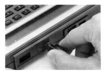
To remove the wand, push down on the button on top of the plug while pulling the plug out.
