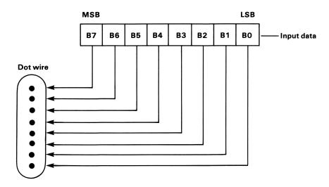
If a bit is "1", the dot is printed; if it is "0", the dot is not printed. For example, assume that the data consists of the ASCII characters " and P:
