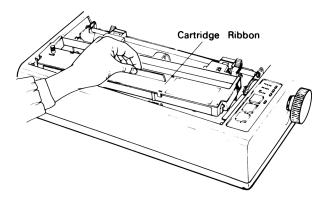
4. Place the ribbon between the printing head nose and the ribbon mask. Do this by turning the ribbon feeding knob on the cartridge case in the direction of the arrow while depressing the ribbon with a pencil (or similar tool).
