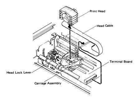
If, for some reason, the print head must be replaced, use the following procedure:
