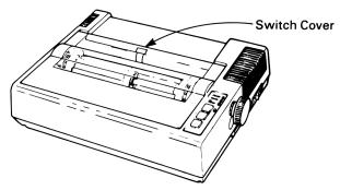
The individual switch segments can be independently set to the ON or OFF position labeled on the switch with the tip of a pencil or similar tool. The ON position of each segment corresponds to binary 1 and the OFF position corresponds to binary 0. Segment six is not used so there are 31 (0 through 30) possible addresses. The following table shows the possible switch settings:
