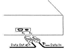
If the drive is the only peripheral to be attached to the controller, you will need only two HP-IL cables. Connect one end of each cable to the drive and the other end to the controller.
