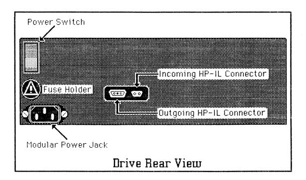
When the drive is turned on, the motor(s) will operate for a few seconds and the drive will perform a self-test to check for proper operation (technical users may wish to refer to Retrieving Drive Status). When the motor stops, you may insert a disk and begin using the drive.
