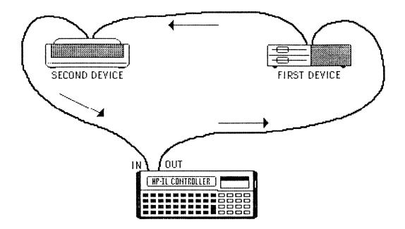
The cables cannot be connected incorrectly but be certain that both ends of a cable are <u>not</u> connected to the same device.
