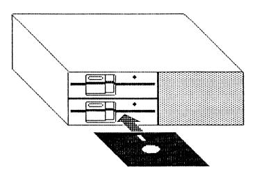
Once a disk has been inserted into the drive and the locking lever turned down to the vertical position, the drive will be ready for use.
