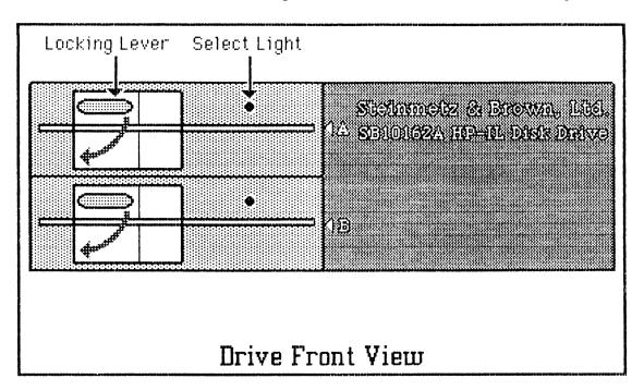
Before Disks can be inserted or removed, the locking lever on the front of the drive must be in the horizontal position.
