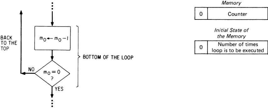
Fig. 1-3 Flowchart for the bottom of a loop
