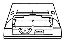
Select either empty port for the Advanced Pocket Professional <sup>™</sup> card, and position the card just outside the slot. Point the triangular arrow on the card toward the HP 48SX port opening, as shown below:
