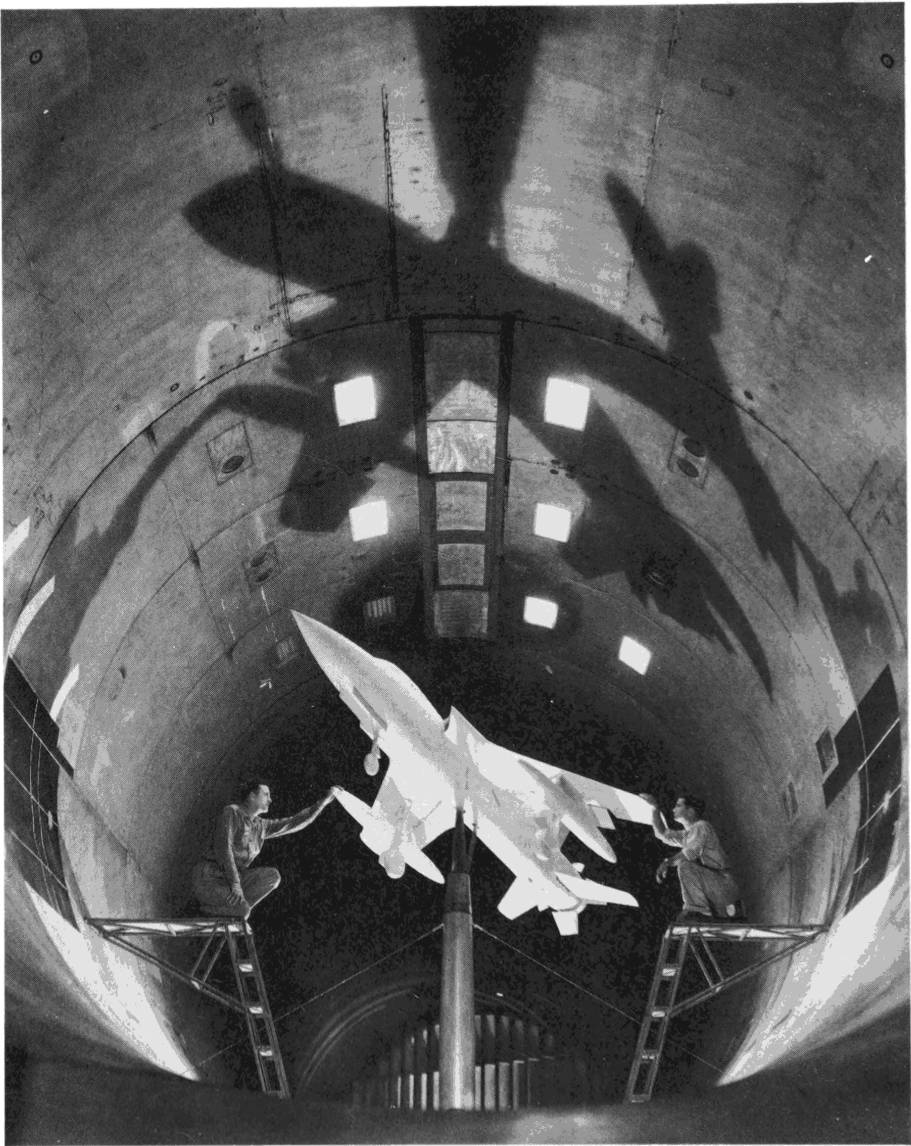
Illustration 5-1. Scale models of the design are frequently tested to prove the validity of the engineer's calculations. Instrumentation on the model pictured above is given a final check by two aircraft technicians prior to testing in the Transonic Dynamics Tunnel. (Courtesy NASA [National Aeronautics and Space Administration.] )
