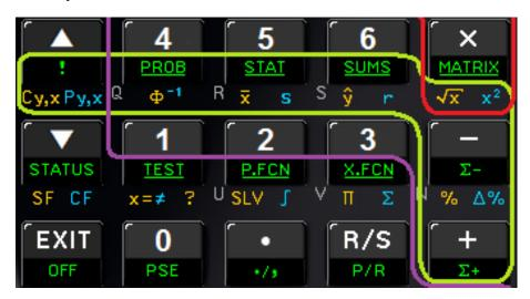
The shifted functions of **4** cover statistical distributions: standard normal **(\Phi**) and its inverse **(\Phi^1**), as well as the catalog **(PROB)** covering nine more continuous distributions and three discrete ones. All these functions have a few features in common:
