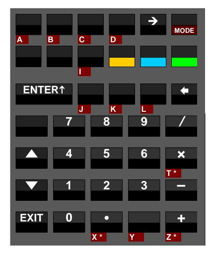
This kind of picture is called a virtual keyboard since deviates from the physical (or real) one of your WP 34S. In such a picture, dark red background is used to highlight changed key functionality. White print denotes primary functions also virtual keyboards, such as the top left key entering the letter A in  $\alpha_{\tau}$  mode directly. On the other hand, what is printed white on your physical WP 34S is called a default primary function.
