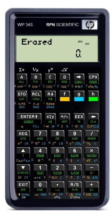
Look at <u>the keyboard of an HP-42S</u> for comparison. The most striking difference to it is the colorful surface of your WP 34S. You get five functions per key on average. White print on key top is for the *primary* function of the key. For secondary functions, green labels are put on the slanted lower faces of 34 keys, golden and blue labels are printed below them on the key plate. Grey letters are bottom left of 26 keys.
