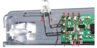
Solder the formerly longer diode leg to terminal 1. Solder the other one to terminal 2.
