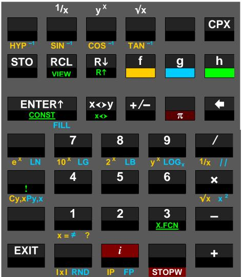
After pressing **CPX**, your *WP 34S* allows for the complex operations shown on this *virtual keyboard* (but STOPW represents an application in real domain, see p. <u>145</u>).
