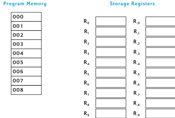
As you key in a 310th instruction, storage register R<sub>0,9</sub> is automatically converted into seven new lines of program memory. The instruction you key in is stored in program line 310, and the instruction `GTO000` is automatically stored in program lines 311 through 316.
