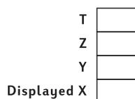
The number in the X-register – and, for two-number functions, the number in the Y-register – are the number(s) used in calculations. The Z- and T-registers are used primarily for the automatic retention of intermediate results during chain calculations, as described in section 1.
