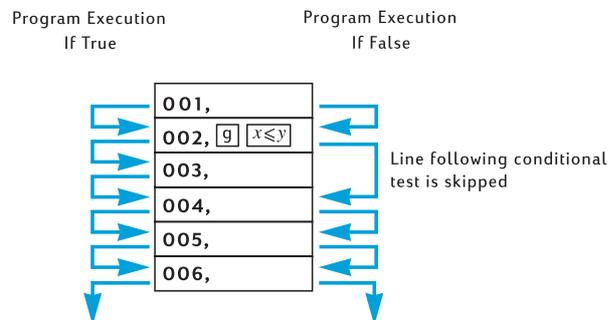
The program line immediately following that containing the conditional test instruction can contain any instruction; however, the most commonly used instruction there is  $\boxed{\text{GTO}}$ . If a  $\boxed{\text{GTO}}$  instruction follows a conditional test instruction, program execution branches elsewhere in program memory if the condition is true and continues with the next line in program memory if the condition is false.
