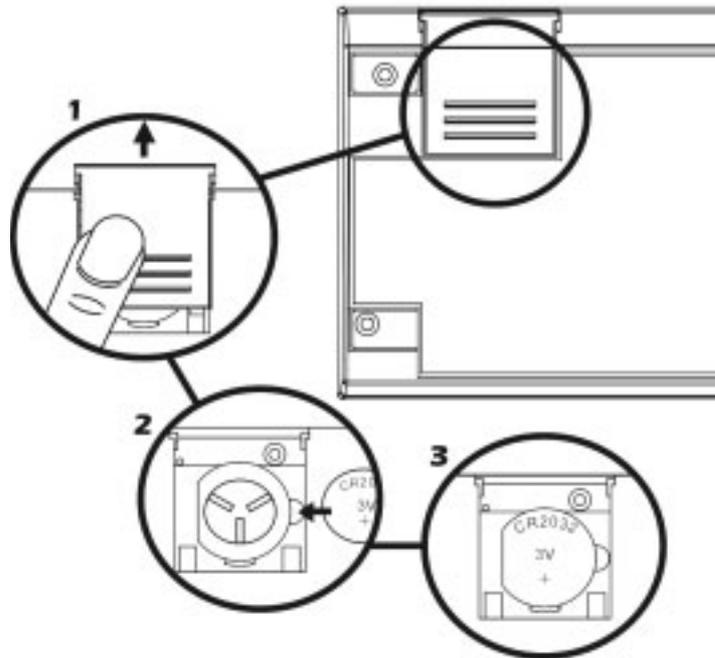
1. With the calculator turned off, slide the battery cover off.
