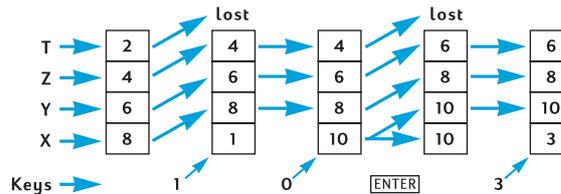
When a digit is keyed into the display, it is simultaneously entered into the X-register. As additional digit keys are pressed, the corresponding digits are appended (that is, added to the right of) those already in the displayed X-register until ENTER is pressed. As shown in the preceding diagram, pressing ENTER does the following:
